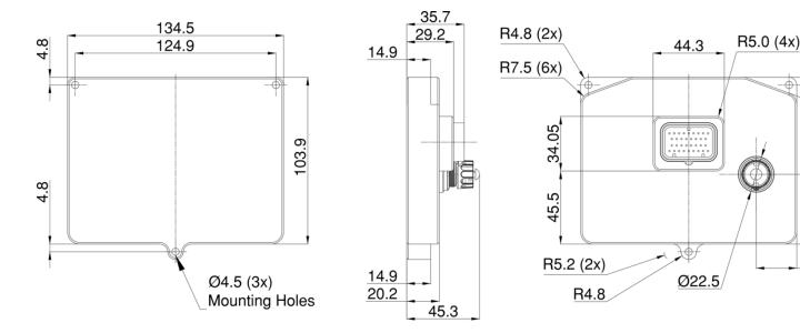
Note: Do not remove any part of the casing. The case provides electromagnetic screening to avoid interference with other equipment, and is also essential for thermal management. Thermal management may be compromised if mounted in a confined space, refer to the operating specifications.
